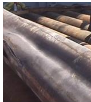
Fig. 1 Casing collapse sample (courtesy of SPE 89775-MS) 1
